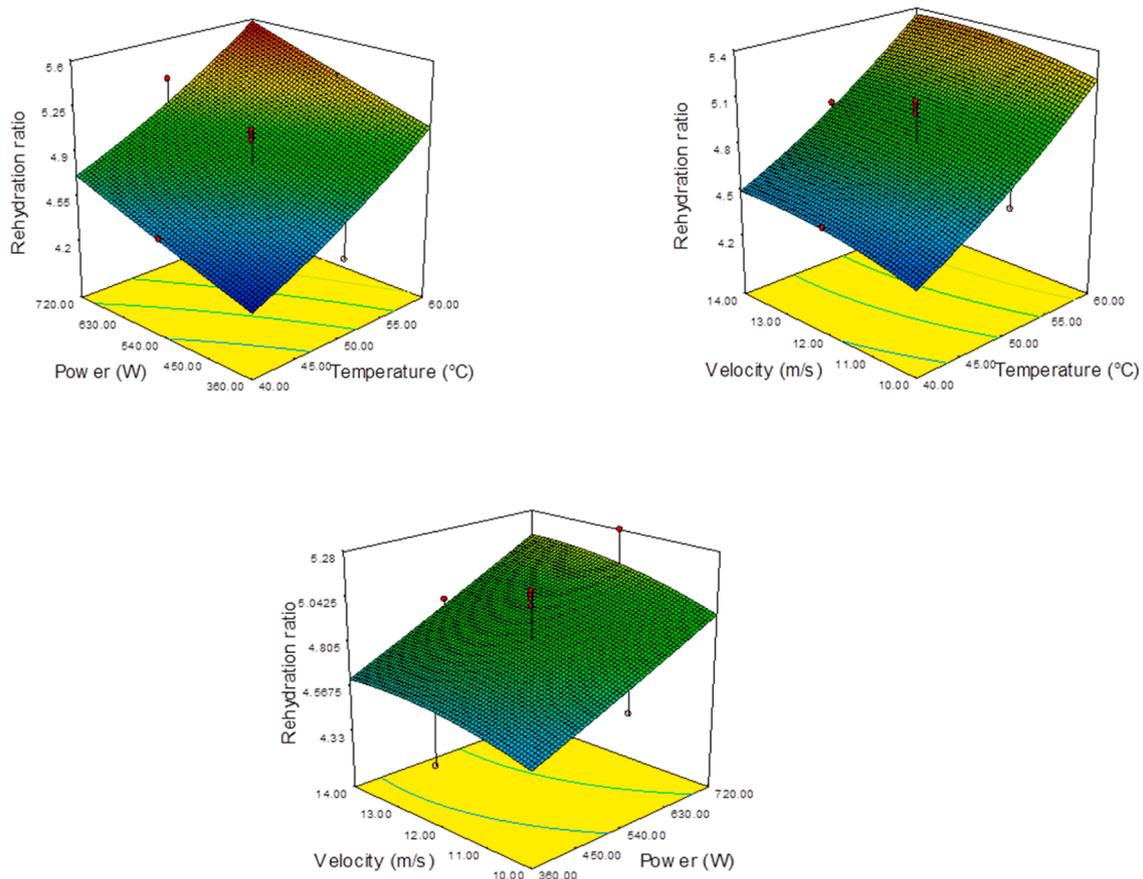
Fig. 2g. Response surface plots showing combined effect of microwave power, temperature and inlet air velocity) on rehydration ratio.
