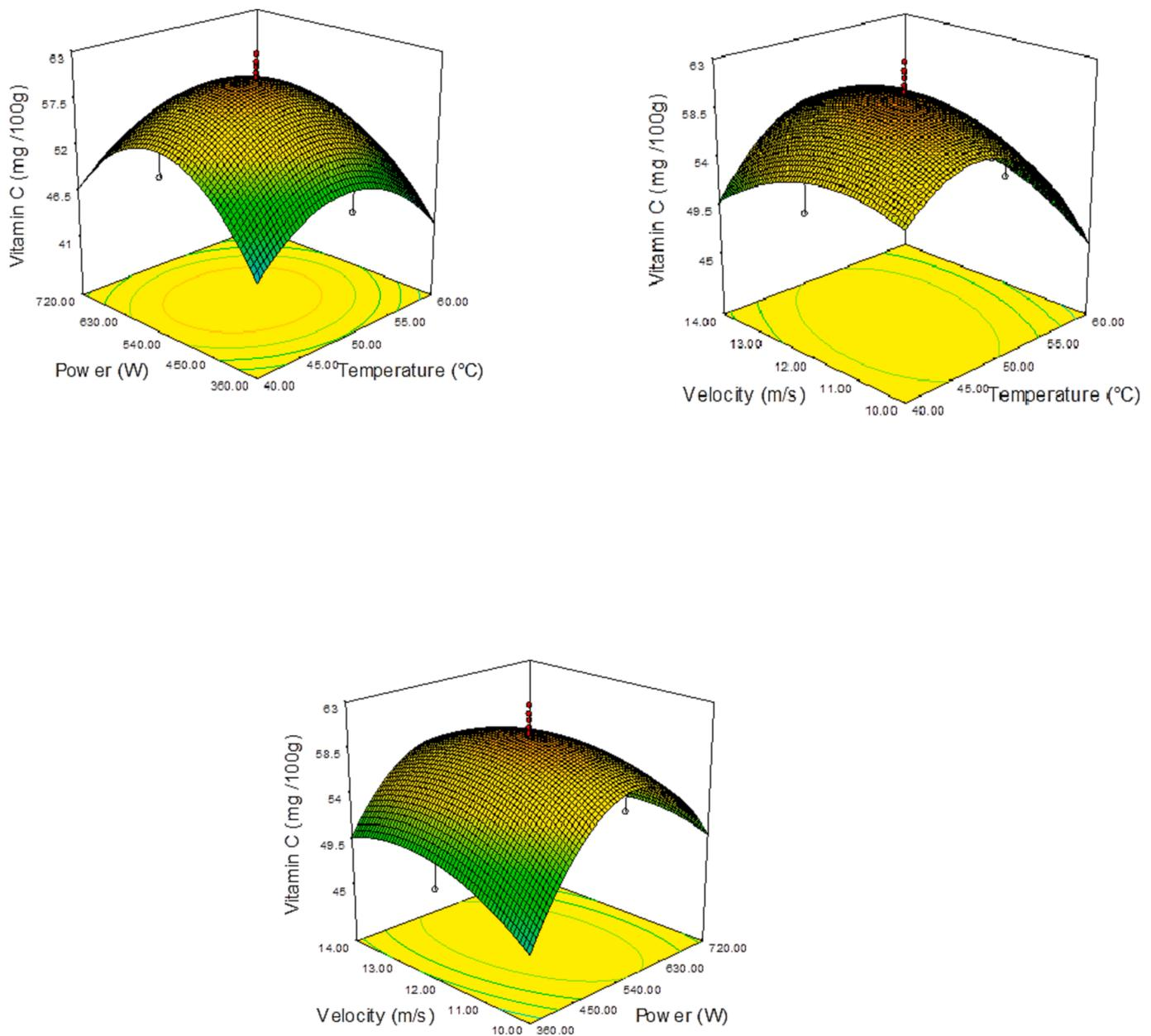
Fig. 2a. Response surface plots showing combined effect of microwave power, temperature and inlet air velocity) on ascorbic acid content.
