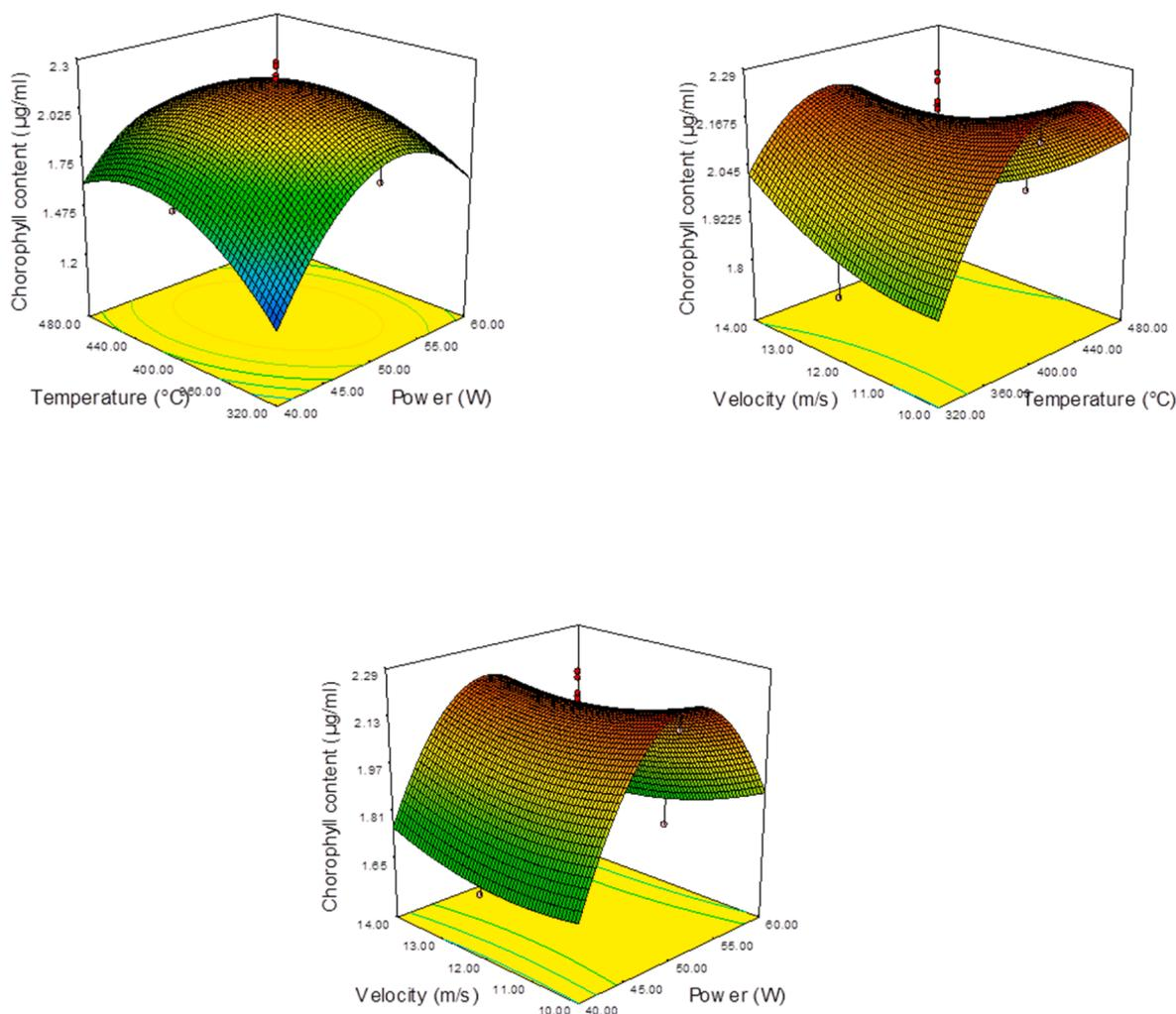
Fig. 2e. Response surface plots showing combined effect of microwave power, temperature and inlet air velocity) on chlorophyll content.
