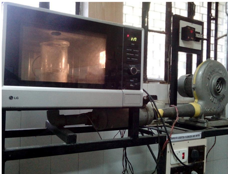
Fig. 1. Experimental apparatus (Microwave assisted fluidized bed drying system) (a) schematic diagram (b) in a working condition.
