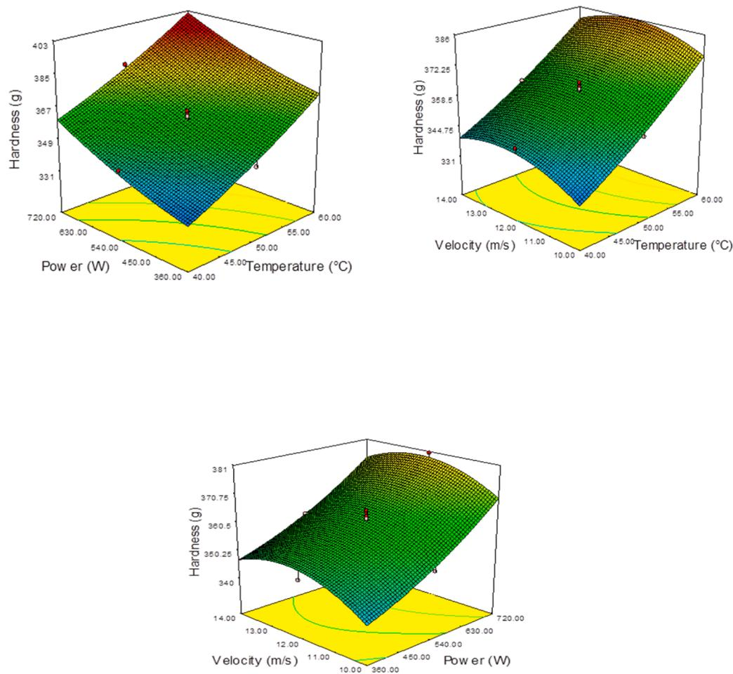
Fig. 2h. Response surface plots showing combined effect of microwave power, temperature and inlet air velocity) on hardness.
