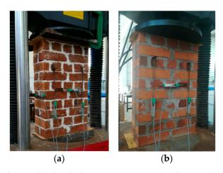
**Figure 2.** (a) Testing of natural hydraulic lime (NHL) mortared wallettes and (b) Testing of ordinary Portland cement (CM) mortared wallettes.
