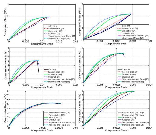
Figure 5. Comparison of experimental and analytical envelop curves.
