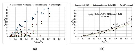
**Figure 6.** Comparison of experimental and analytical plastic strains (**a**) Mendola and Papia [35], Sema et al. [27] and Crisafulli [26] and (**b**) Facconi et al. [28] and Subramaniam and Sinha [25].
