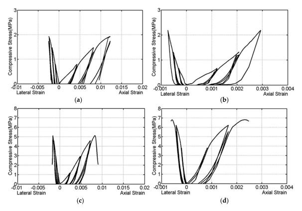
**Figure 4.** Cyclic compressive stress–strain curves of the wallettes under compression (a) CB1-NHL, (b) CB1-CM, (c) CB2-NHL, and (d) CB2-CM.
