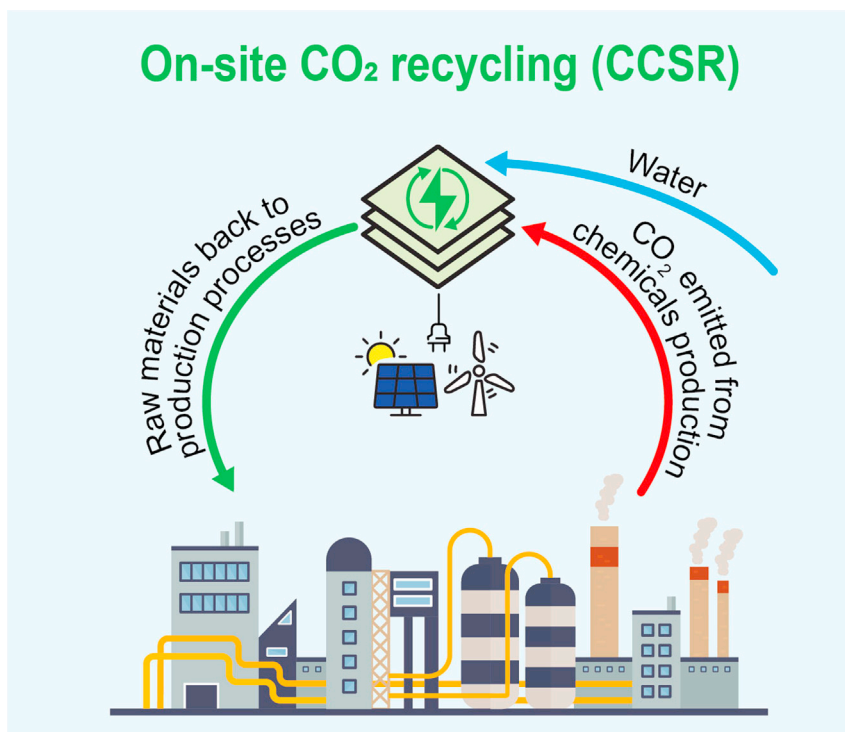
Figure 2. Conceptual depiction of Carbon Capture On-Site Recycling (CCSR): CO 2 emissions from a chemical plant, usually vented to the atmosphere, are instead sent to a CO 2 R reactor and converted to products reverted to the main production process, all in the same chemical plant
