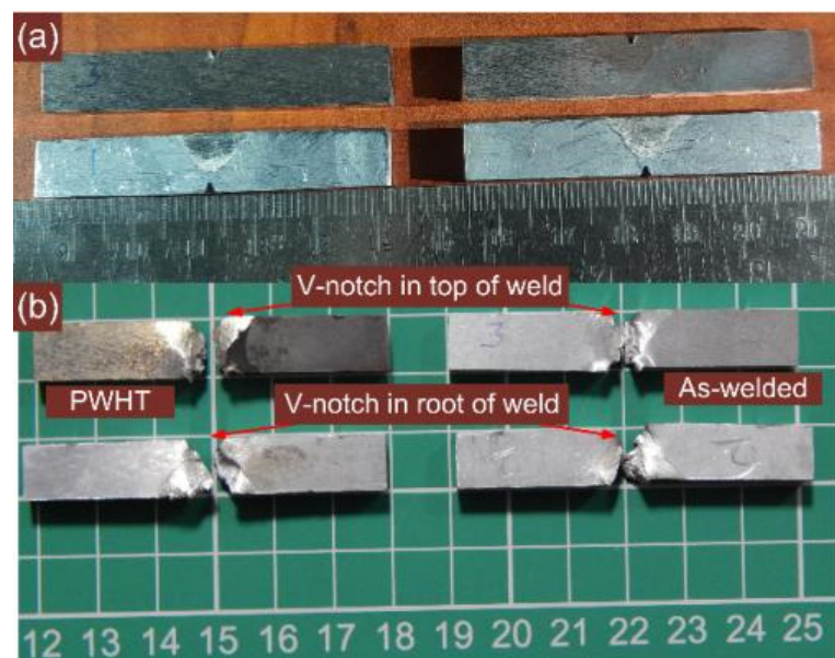
Figure 16. (a) Position of notch in top and bottom portion, (b) fractured impact toughness specimen for the weld metal.
