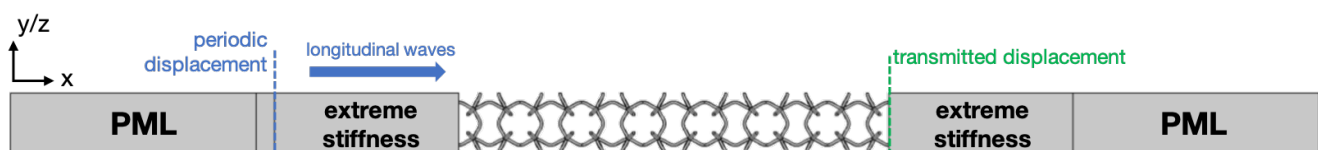
Figure 3. Setup for the transmission simulation. Longitudinal waves are transmitted from left to right. The excitation of the waves is guaranteed to be perfectly longitudinal by domains of extreme stiffness. Perfectly matched layers (PMLs) prevent artifacts from reflections. The transmitted displacement is evaluated at the interface between the cellular array and second extreme stiffness domain. Periodic conditions are applied in y - and z -direction.
