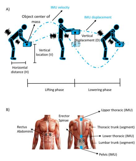
**Figure 1.** (**A**) description of the experimental setup and of the lifting cycle: displacement and velocity of the IMU placed on the load were used to define the lifting and lowering phases (see Section 2.5.1 for further details). (**B**) Locations of the IMU (blue squares) and sEMG (white circles) electrodes.
