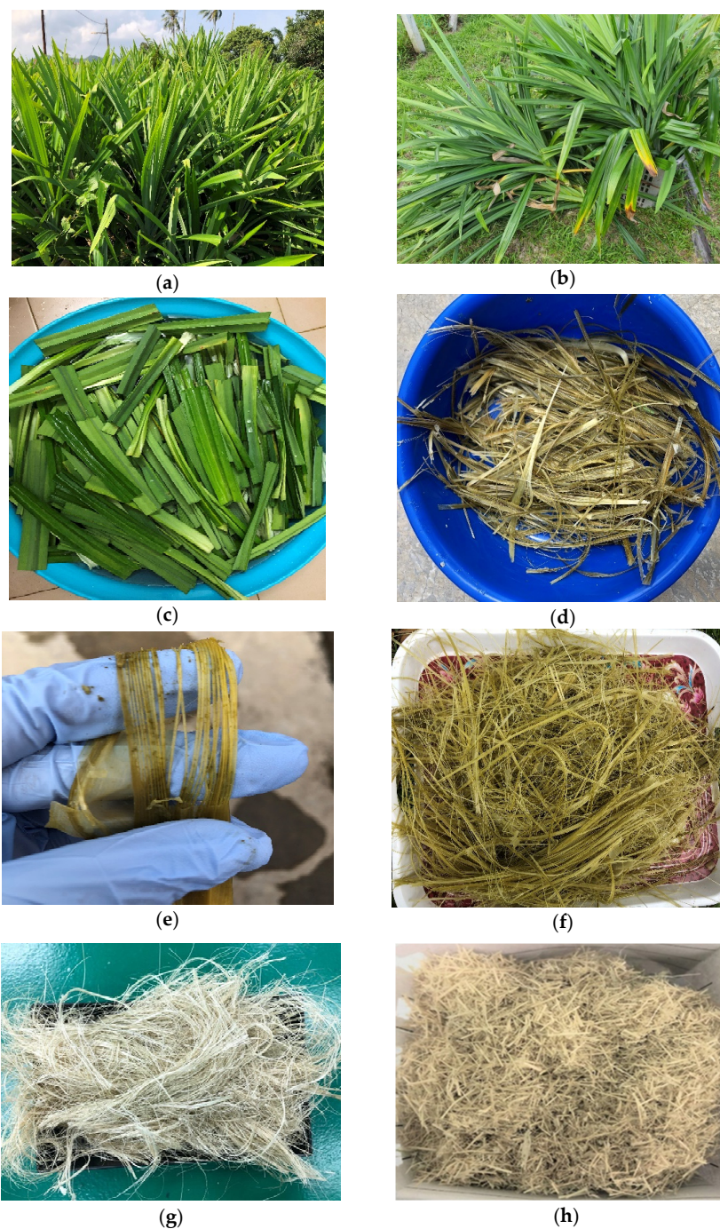
Figure 1. Pictorial view of fibre extraction (a) Pandanus amaryllifolius plant; (b) cut bulk of leaves; (c) leaves cleaned and immersed in the water; (d) after 2 weeks; (e) skin degraded and removal of fibres; (f) extracted fibres collected and dried under sunlight; (g) ungrounded fibres after being further dried in oven; (h) ground (short fibres) PAF.
