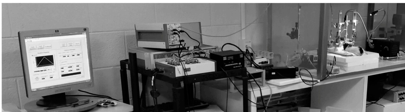
Figure 1. Modern FSCV set up for the in vivo monitoring of extracellular dopamine in the rodent brain. The voltammetry data collection hardware and software were developed in Electronics Design Facility at University of North Carolina at Chapel Hill. FSCV system is combined with the equipment for optogenetic experiments via TTL signal.
