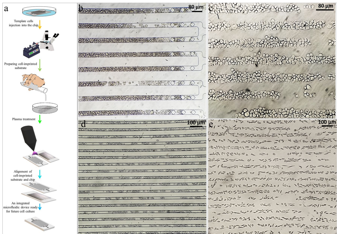
Figure 5. (a) The schematic of the cell-imprinted-based integrated microfluidic device fabrication procedure. (b) The function of the microfluidic chip in trapping the HUVEC cell line in an area around terminal microposts of 40 μm microchannels of the microfluidic chip, which is almost filled with cells after injection with a syringe pump. (c) The regular pattern of HUVEC cell lines transferred to the cell-culture plate. (d) 25 μm microchannels of the microfluidic chip are almost filled with L929 cell line after injection with a syringe pump. (e) The regular pattern of L929 cell lines transferred to the cell-culture plate.
