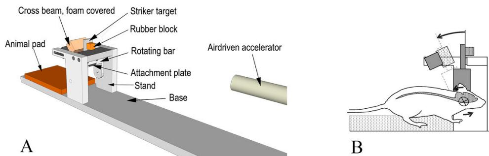
**Figure 1.** Experiment setup scheme. (A) Oblique view of the test device. (B) Side view of the test subject placed within the device. The central nervous system (CNS) is schematically depicted, and the center of rotation highlighted. The arrows indicate the direction of movement.
