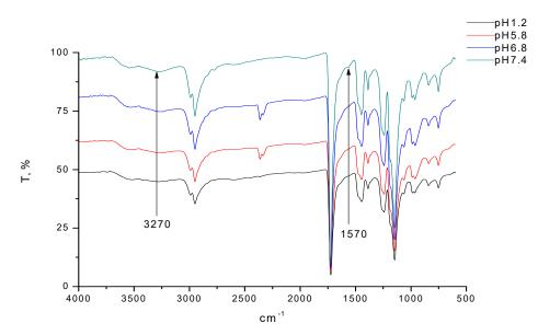
**Figure 6.** FTIR-spectra of polycomplex compacts (prepared from IPC-1), after swelling in buffer solutions mimicking the pH values in different parts of gastrointestinal tract.
