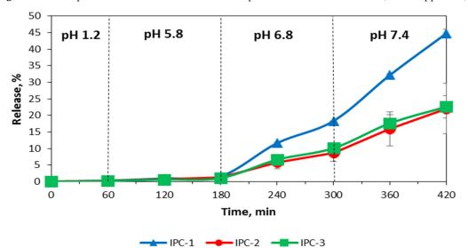
**Figure 9.** Release profiles of indomethacin from IPC compacts in the buffer solutions mimicking the environment of gastrointestinal tract (USP III apparatus).
