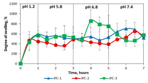
Figure 5. Swelling profiles of IPC compacts in buffer solutions mimicking the pH values in different parts of gastrointestinal tract.
