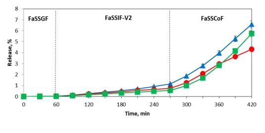
Figure 8. Release profiles of indomethacin from IPC compacts in the biorelevant media (USP IV apparatus).
