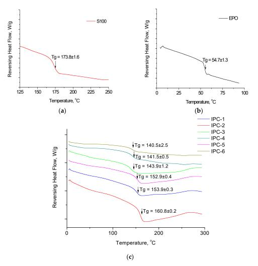
**Figure 3.** Exemplar differential scanning calorimetry (DSC) thermograms of interpolymer complexes and Eudragit<sup>®</sup> copolymers: (**a**) Eudragit<sup>®</sup> S100; (**b**) Eudragit<sup>®</sup> EPO and (**c**) IPCs.
