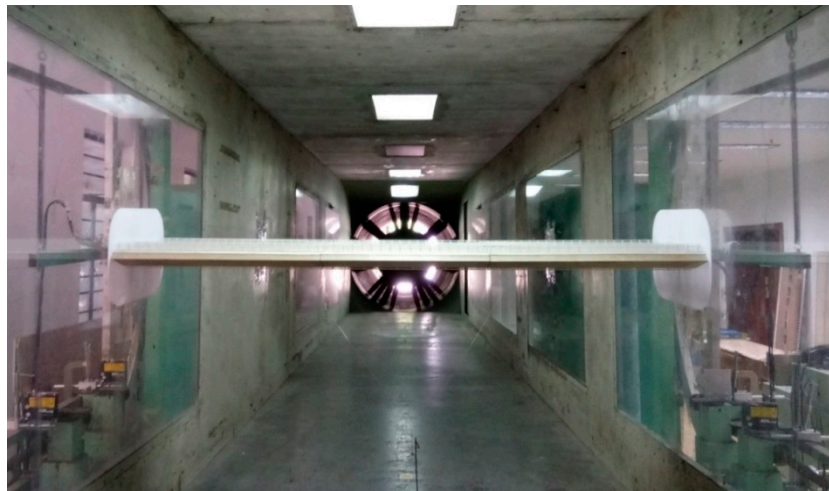
Figure 1. View of the spring-suspended sectional model in TJ-1 wind tunnel.
