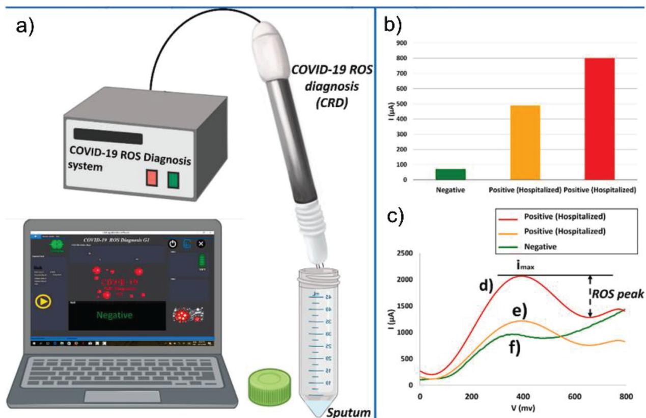
**Figure 5.** (a) COVID-19 ROS diagnosis (CRD) system consists of three needle electrodes coated with functionalized multiwall carbon nanotubes. (b) Selective electrochemical reactions of released ROS on MWCNTs produces cathodic ionic peaks. (c) ROS-related electrochemical cyclic voltammetry cathodic peaks from the fresh sputum of two different patients were involved in COVID-19 and hospitalized in comparison with a confirmed normal case. (Reproduced with permission from ref 92. Elsevier Ltd.)
