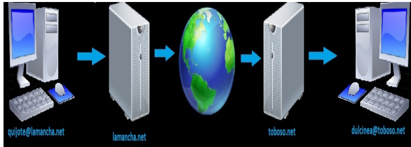
Figure 4. Connection process between two users via the Extensible Messaging and Presence Protocol (XMPP).
