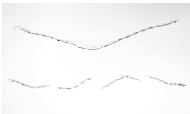
Fig. 4. Results of the in vitro maximal stretching test of two different types of stents. (A) is the stent with 3 connectors (Xience Xpedition, Abbott Vascular, Santa Clara, CA, USA) that was not fractured but rather elongated. (B) is the stent with 2 connectors (Promus Premier, Boston Scientific, MN, USA) that was fractured into four segments.
