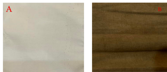
Figure 1. (A) Non-coated cotton fabric and (B) cotton fabric coated with CuO nanoparticles.
