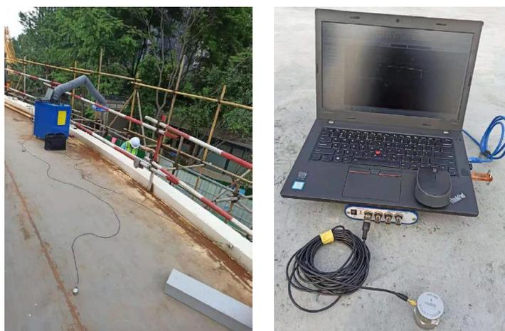
**Figure 2.** Instrumentation of the investigated pedestrian bridge with accelerometers.
