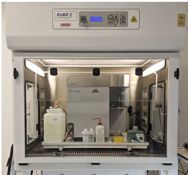
FIGURE 3 Example placement of a 3-laser benchtop analyzer inside a Class II Biological Safety Cabinet [Color figure can be viewed at wileyonlinelibrary.com ]
