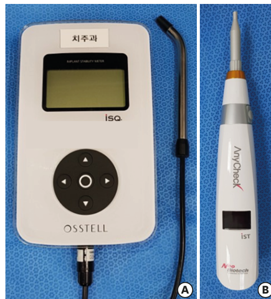
Figure 3. Implant stability analysis devices. (A) Resonance frequency analysis device. (B) Damping capacity analysis device.
