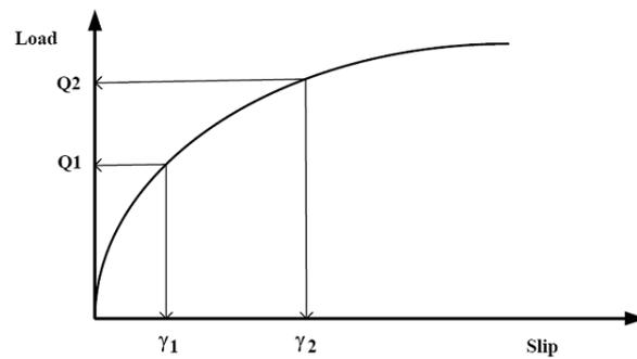
Figure 2. Typical load-slip relationship from the standard test.
