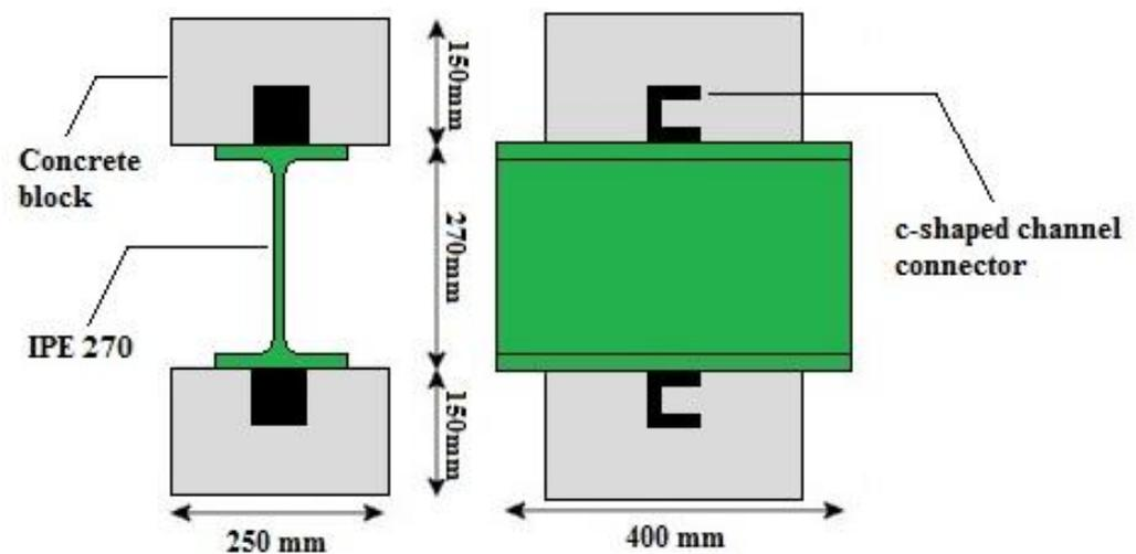
Figure 1. Schematic view of the test specimen.
