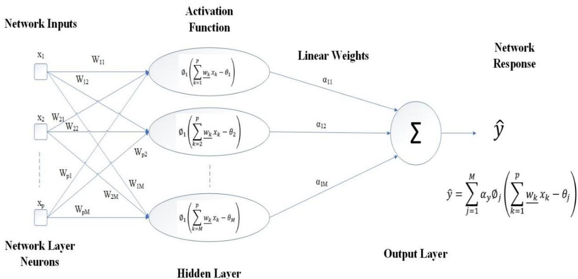
Figure 15. Flowchart of typical single line hidden layer MLP for identifying a problem.
