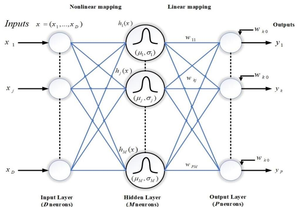
Figure 19. The architecture of an RBF network.
