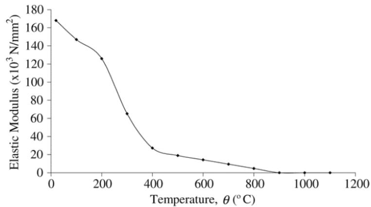
Figure 7. Modulus of elasticity of structural steel at elevated temperatures, EC3 British Standards Institution.
