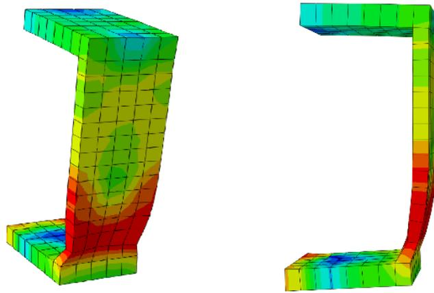
**Figure 11.** Typical channel connector failure at elevated temperature.
