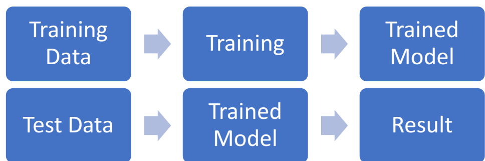
Fig. 7 The validation of prediction model. The validation process is illustrated. The accuracy of the trained model is verified by testing it over partitioned test data
