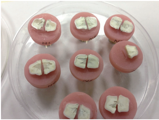
Fig. 1. Sectioned copings mounted in acrylic resin.
