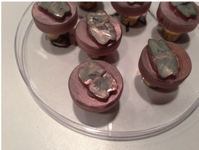
Fig. 2. Sectioned copings coated with fine coat ion sputter JFC-1100.
