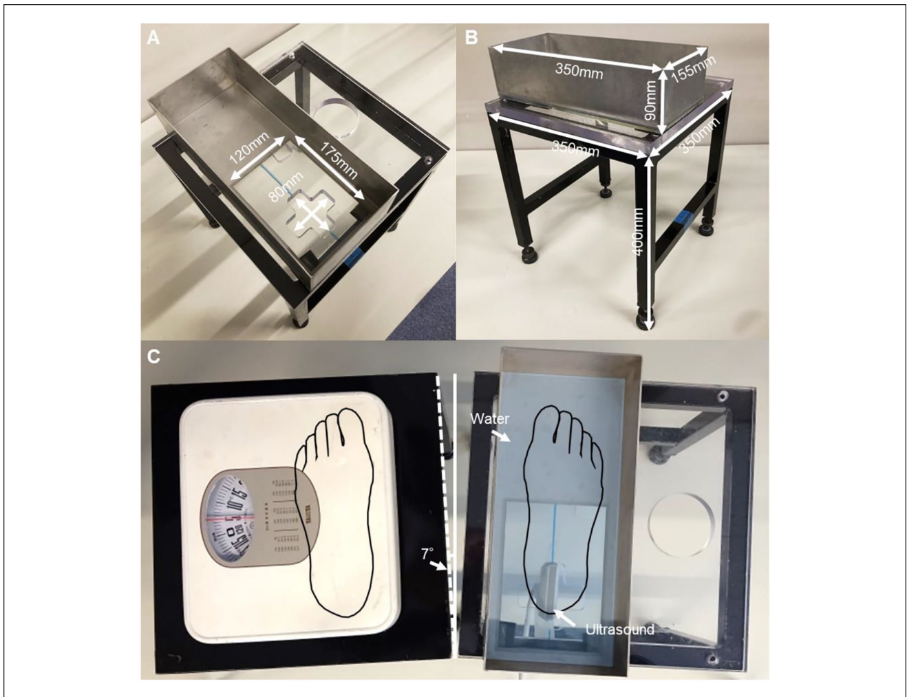
Figure 1. Load-measuring instrument. (A and B) Load-measuring instrument and tank: Lines are drawn on the weightbearing device to indicate where to place your feet. A water tank was placed along the drawn line, and the subjects were instructed to place the second metatarsal bone and calcaneus bone on the line. A fixture was attached to the measurement surface to prevent the water tank from moving during unloading operations. (C) Position of the foot on the load device: The right foot was immersed in water, and observations were made using an ultrasonographic imaging diagnostic device through the cross-shaped hole created in the heel area.
