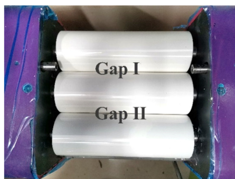
Figure 1. The three rollers and two gaps of a three-roll milling machine.
