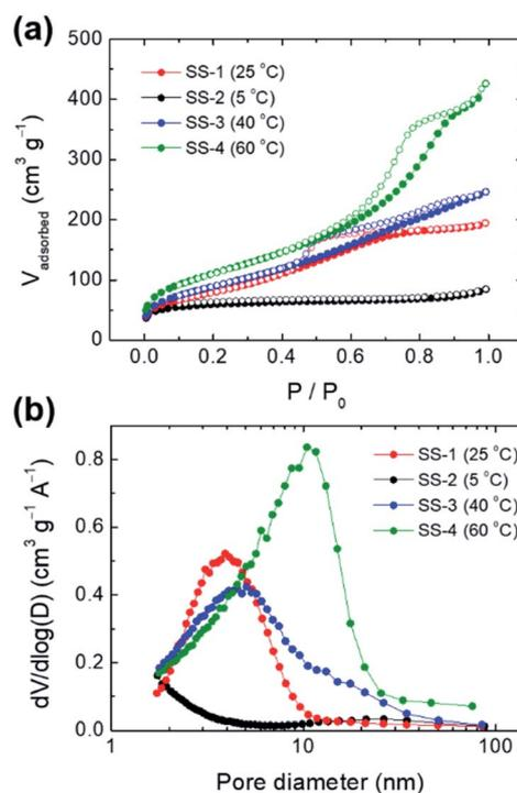
Fig. 7 (a)  $\text{N}_2$  physisorption isotherms and (b) pore size distributions of SS-1 (25 °C), SS-2 (5 °C), SS-3 (40 °C), and SS-4 (60 °C). Each value in parentheses represents the temperature of the precipitation process.
