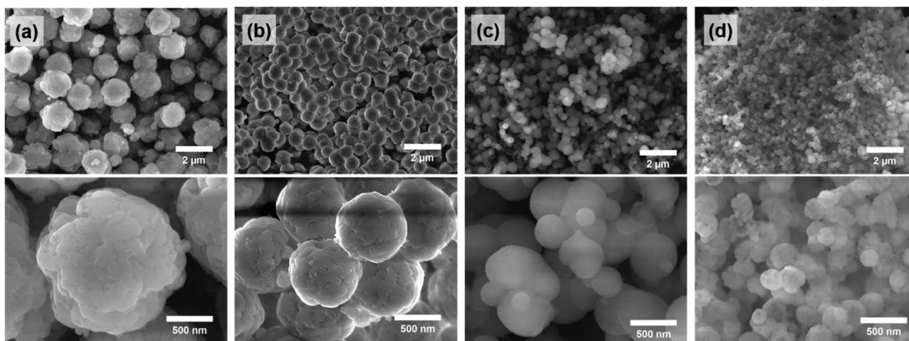
Fig. 6 SEM images of (a) SS-2 (5 °C), (b) SS-1 (25 °C), (c) SS-3 (40 °C), and (d) SS-4 (60 °C). Each value in parentheses represents the temperature of the precipitation process.
