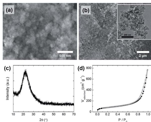
Fig. 5 (a and b) SEM images (inset: TEM image), (c) XRD pattern, and (d) N<sub>2</sub> physisorption isotherms of silica particles (S-2), synthesized using a silicate solution extracted under harsh conditions.
