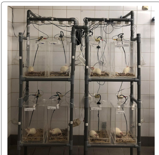
Fig. 3 EEG rack system. Each rack houses 4 cages, two on each shelf. Every 2 racks (8 cages) are monitored by one EEG recorder. We built a rack system that does not contain metal or other conductive material which provides the simplest and most efficient technique to electrically isolate rats from each other and from environmental sources of electricity. This has markedly contributed to minimizing electrical artifact, which is a challenge commonly faced when simultaneously recording multiple animals
