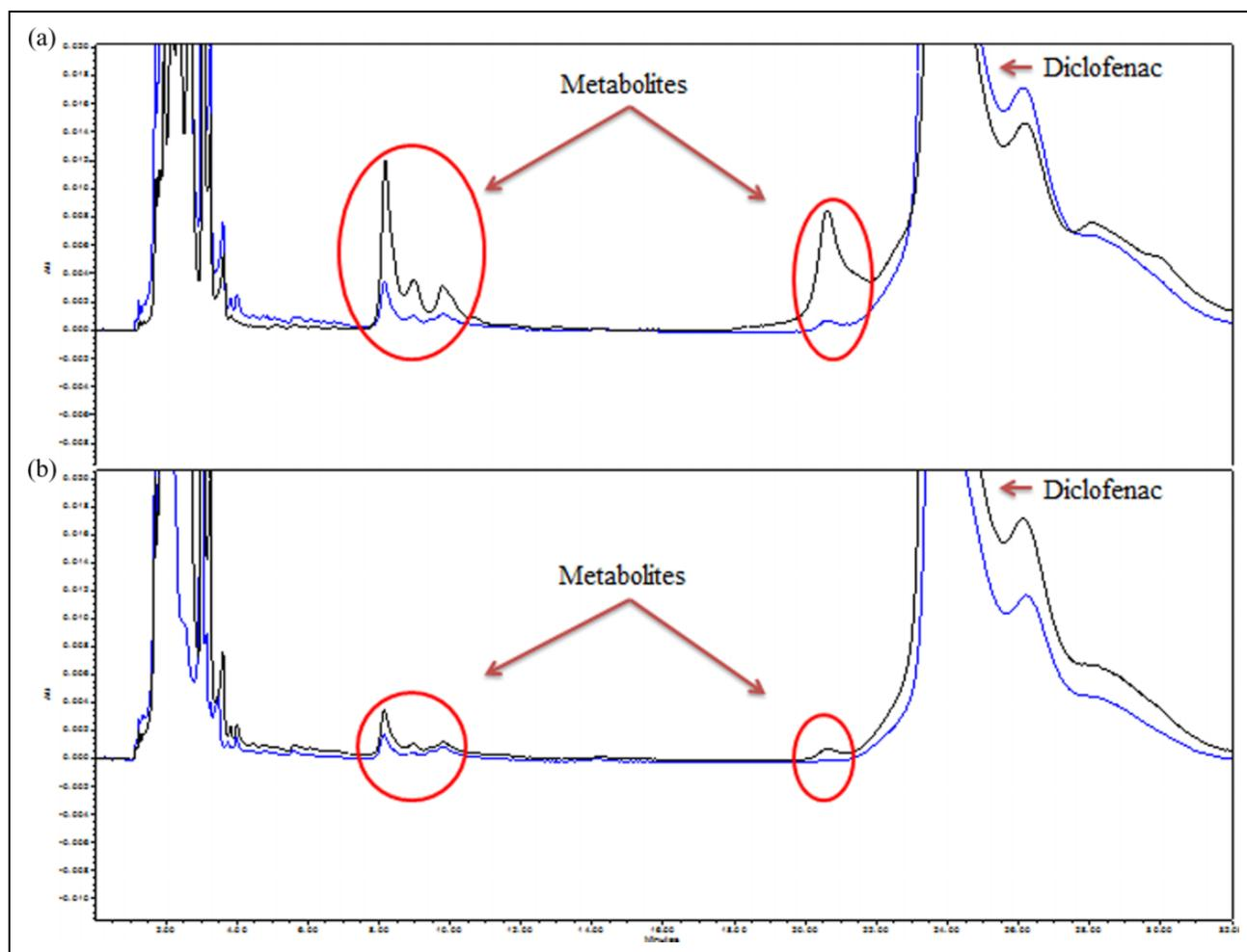
**Figure 6.** HPLC chromatograms of diclofenac metabolization with *online* injection. (a) shows the *online* result (in blue) compared to control situation in culture flask: adherent cells (in black). (b) compared the metabolization into the analytical bioreactor between *online* (in black) and *off-line* injections (in blue). HPLC: high-performance liquid chromatography.
