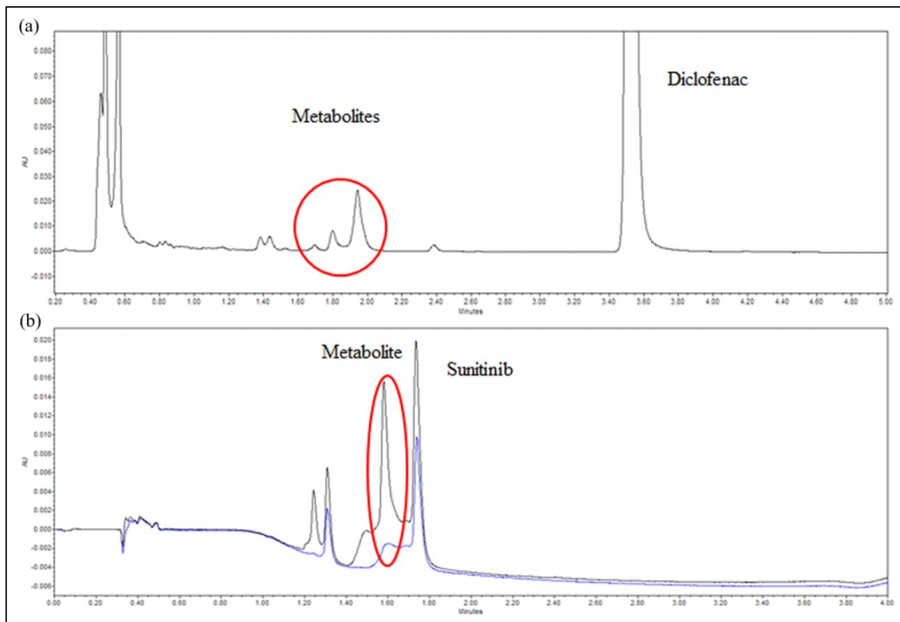
**Figure 4.** Generated UPLC chromatograms after drug metabolization of magnetically immobilized cells into our holder. (a) represents the 250  $\mu\text{M}$  diclofenac metabolization sample. (b) shows the 20  $\mu\text{M}$  sunitinib metabolization sample after tubing desorption by methanol (in blue) and the tubing control desorption sample of 20  $\mu\text{M}$  sunitinib and *N*-desethyl sunitinib (in black).
