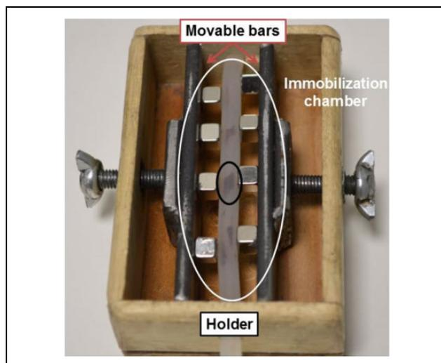
**Figure 1.** Picture of the immobilization bars chamber (8 × 5 × 3 cm). The two iron bars can be moved by screws in order to modify the distance between the magnets and the silicone tubing. Labeled HepaRG cells are magnetically stopped in front of the magnets (dark circle).
