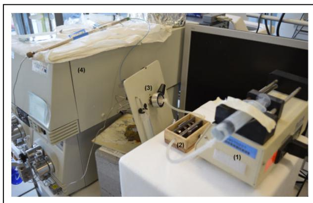
**Figure 5.** Online metabolization test design: (1) syringe pump, (2) wooden magnet holder, (3) Rheodyne injection valve, and (4) HPLC system. HPLC: high-performance liquid chromatography.
