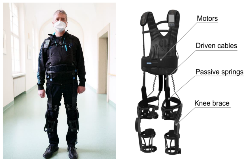
Figure 1 The Myosuit—an exoskeleton-type robotic device.
