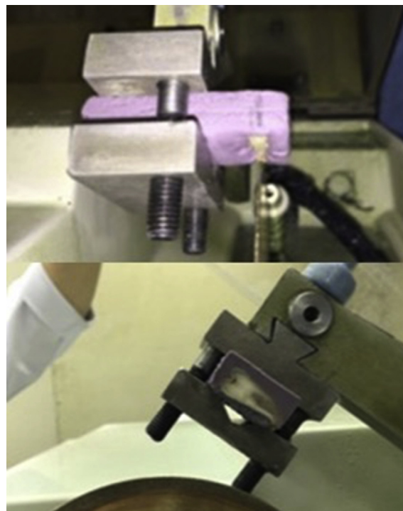
Fig. 2 Tooth mounted, prepared for sectioning Procedures, and cross-sectional part of the tooth structure.
