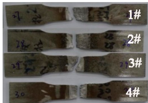
Figure 9. Fracture locations of flat tensile specimens with different treatments methods: 1—untreated; 2—pneumatic chipping hammer; 3—ultrasonic peening treatment; 4—heat treatment.
