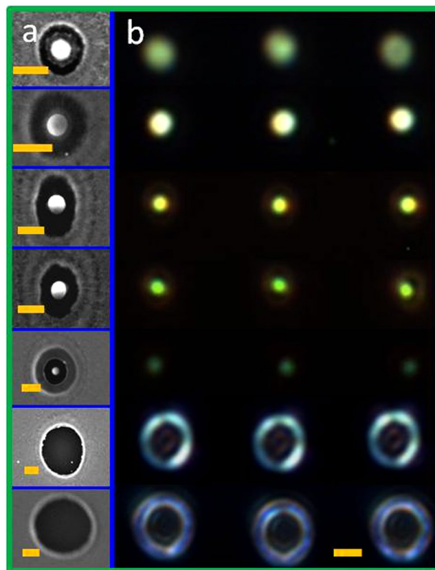
Figure 6. (a) SEM images (scale bar, 500 nm) of nanostructures fabricated from 40-nm-thick Au film at slightly different laser pulse energies of 0.021, 0.022, 0.023, 0.024, 0.025, 0.032, and 0.034 \mu\text{J} from top to bottom in each line. (b) Changes in the optical responses of the nanostructures are visualized by DF microscopic images (scale bar, 5 \mu\text{m} ).
