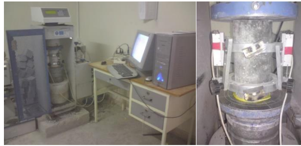
Figure 3. Compressive strength stress-strain tests apparatus.
