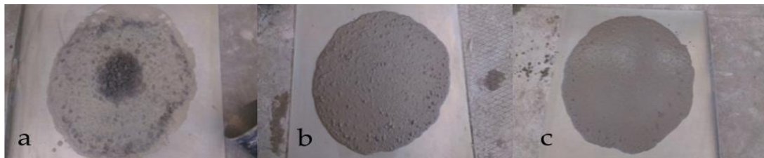
Figure 4. Concrete mixtures prepared with recycled aggregates: (a) concrete mixture without AEA and Sf; (b) concrete mixture with AEA; and (c) concrete mixture with Sf.
