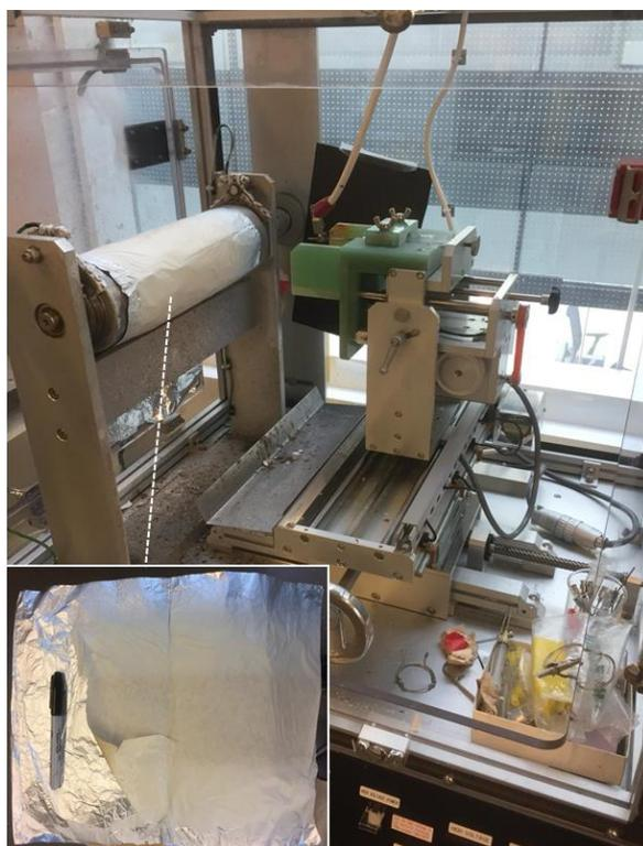
**Figure 12.** Electrospinning apparatus and membranes. Shows the nanofiber electrospinning unit (Kato) and a electrospun PVA membrane (10% PVA (99%):90% PVA (88%)) containing silver carbonate (1%).
