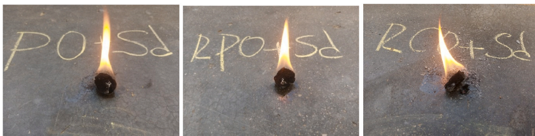
Fig. 5. Burning test of EFS.
