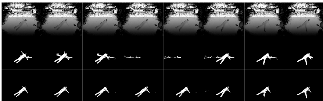
Figure 5. Experimental results of human segmentation. First row is depth images, second row is human segmentation using Kinect SDK and the third row is human segmentation using ETDA-Net.
