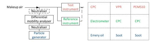
**Figure 2.** Experimental setups for the calibration of the instruments. CPC = Condensation particle counter; PEMS = Portable emissions measurement system; VPR = Volatile particle remover.
