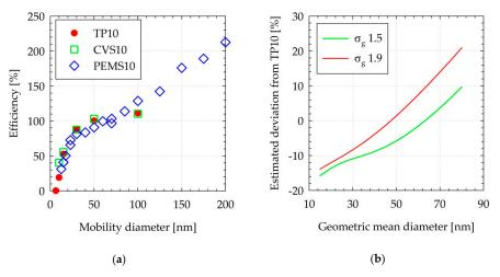
**Figure 3.** (a) Efficiency curves of the systems used at the tailpipe and the dilution tunnel. (b) Simulated deviation between the PEMS10 and TP10 for lognormal distributions of different geometric mean diameters (horizontal axis) and two different standard deviations  $\sigma_g$  (1.5 and 1.9). CVS = Constant volume sampling; PEMS = Portable emissions measurement system; TP = Tailpipe.
