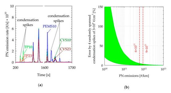
**Figure 8.** (a) Sections of the WLTC test of the CNG vehicle in which condensation-related concentration spikes were detected with the TP10, TP23, and PEMS10. (b) Calculated effect of four randomly spanned condensation spikes of  $3 \times 10^6$  #/cm<sup>3</sup> in the real-time traces of the various vehicles tested. The shaded area corresponds to the maximum and minimum calculated effect. Dashed lines indicate the laboratory and on-road emission limits. Abbreviations as in Table 1.
