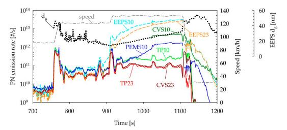
**Figure 9.** Real-time PN emissions and geometric mean diameters over steady-speed ramps of the SIDI vehicle. Abbreviations as in Table 1.
