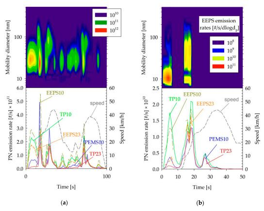
**Figure 6.** Real-time size distributions (top panel) and PN emission rates (bottom panel) over (**a**) the first 100 s of a cold-start WLTC test of the D + DPF vehicle and (**b**) the first 50 s of a cold-start WLTC test of the SIDI + GPF vehicle. Abbreviations as in Table 1.
