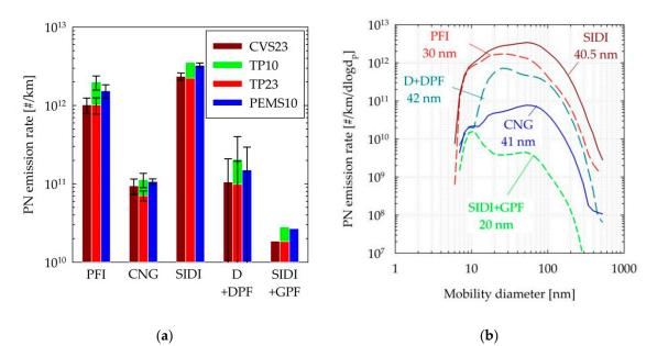
**Figure 4.** (a) Average PN emission rates over the WLTC tests of the different vehicles tested. Error bars correspond to min–max of two tests. (b) Cycle-average size distributions over the WLTC tests. The reported sizes correspond to the geometric mean diameters. Abbreviations as in Table 1.
