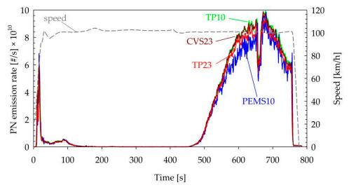
**Figure 7.** Real-time PN emissions during the forced regeneration of the D + DPF vehicle. Abbreviations as in Table 1.
