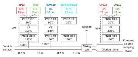
**Figure 1.** Experimental setup of the chassis dynamometer testing. CPC = Condensation particle counter; CS = Catalytic stripper; CVS = Constant volume sampling; DC = Diffusion charger; EEPS = Engine exhaust particle sizer; ET = Evaporation tube; PEMS = Portable emissions measurement system; PND = Particle number diluter; TP = Tailpipe.
