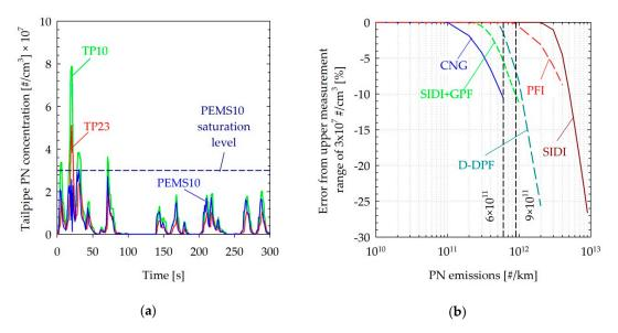
**Figure 5.** (a) Real-time particle number (PN) concentrations at the tailpipe over a cold-start WLTC test of the PFI vehicle. (b) Calculated contribution of the upper measurement range of the PEMS10 on the cycle average emissions for different vehicle technologies. Dashed vertical lines indicate laboratory and on-road PN limits. Abbreviations as in Table 1.
