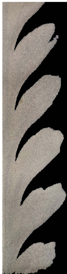
Figure 9. The FSW layer segmentation outcome based on the multi-stage adaptive binarization scheme.
