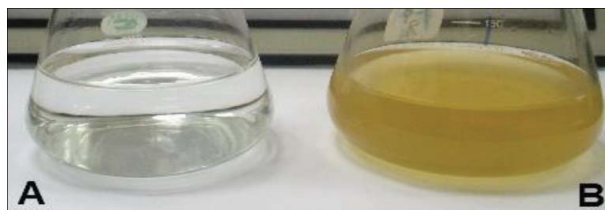
Figure 2. Conical flasks containing the extracellular filtrate of the Cladosporium cladosporioides biomass in aqueous solution of 10^{-3} M \text{AgNO}_3 at the beginning of the reaction (A) and after 1 day of reaction (B).
