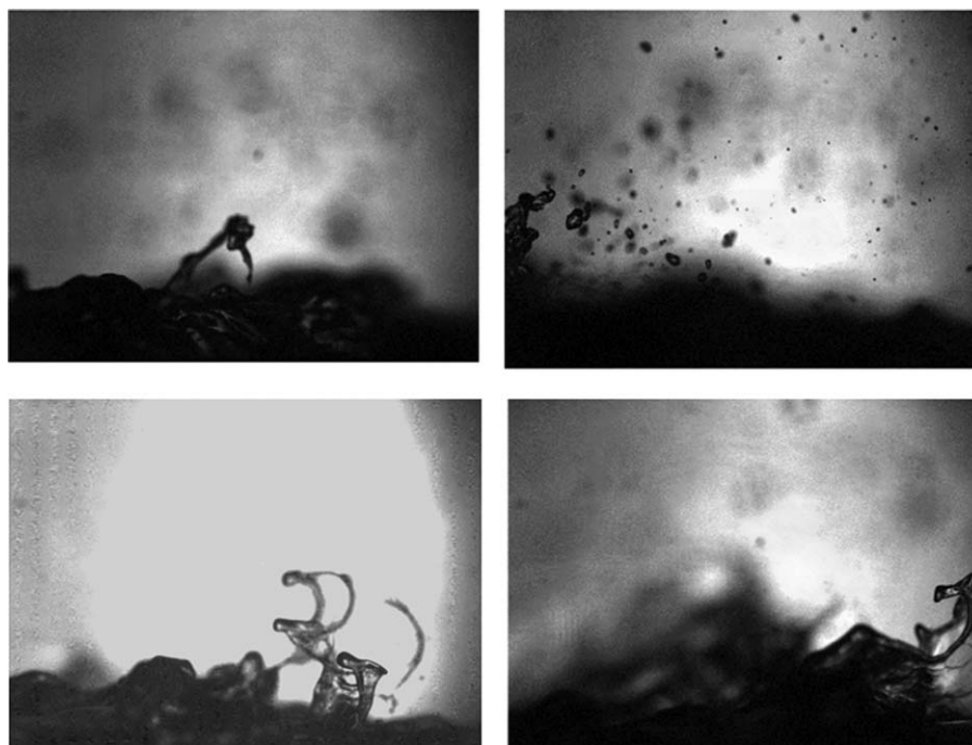
Figure 2. Disruptions of the air-water interface under hurricane-force wind revealed with shadow-imaging techniques. The equivalent wind speed is U_{10} = 40 \text{ m s}^{-1} (equivalent to a Category 2 tropical cyclone). This laboratory experiment was conducted at the UM RSMAS ASIST facility (Soloviev et al., 2014). The large difference in density between the air and water leads to strong asymmetry of the KH instability process (Hoepffner et al., 2011). Note that the shadow imaging technique used for visualization in this experiment could not resolve air bubbles in the water. (top) Finger-type ejection from the surface and (bottom) bag development from looped structures. According to the laboratory experiment conducted by Troitskaya et al. (2017), spray generation by the bag structures dominated over that of the fingers (the laboratory conditions corresponded to a Category 1 storm).
