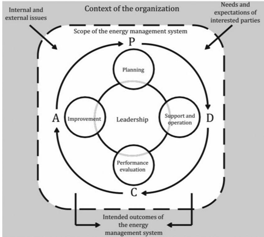
Fig. 3. Plan-do-study-act (PDSA) cycle which know as Deming Cycle of management is a four-step modification process model, used as a technique for project planning.
