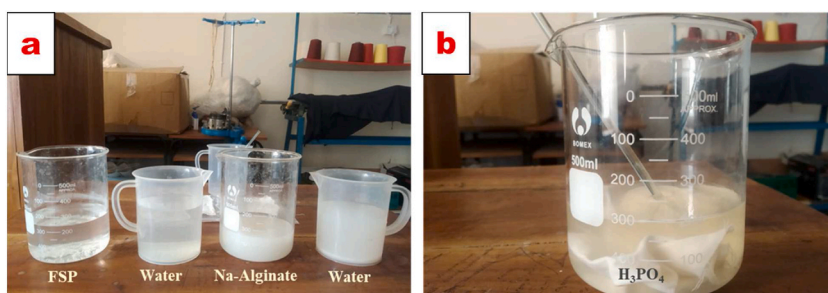
Scheme 2. Layer-by-layer deposition (a) and dipping process of cotton fabric (b).
