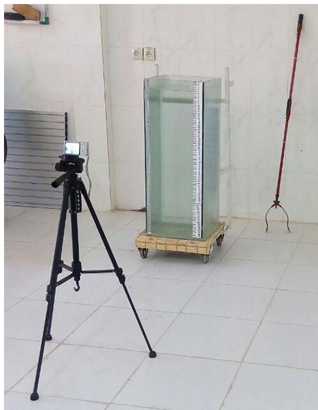
FIGURE 2 Plexiglas column, the clamp, and the position of the camera
