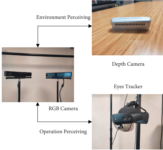
FIGURE 1: Vision system: the combination of fixed cameras and eye tracker.
