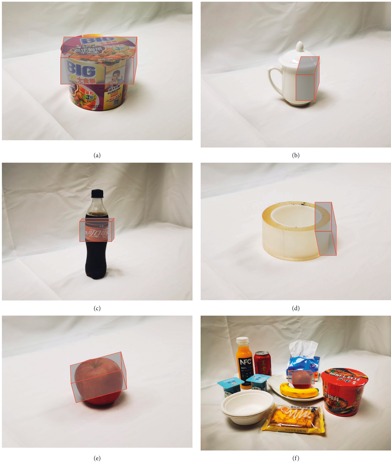
FIGURE 13: Grasp position prediction of single objects and combinations. (a–e) Object grasping position. (f) Combination grasping position.
