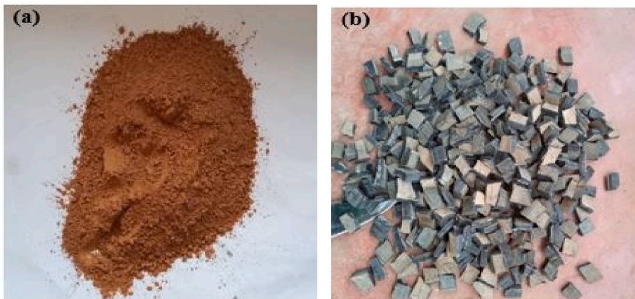
Fig. 2. Generated non-conventional construction materials (a) WCBP (b) WTR.
