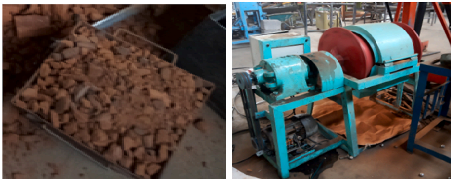
Fig. 1. Process of ball milling: unmilled clay brick fragments (left) and grinding fragmented bricks using ball mill (right).
