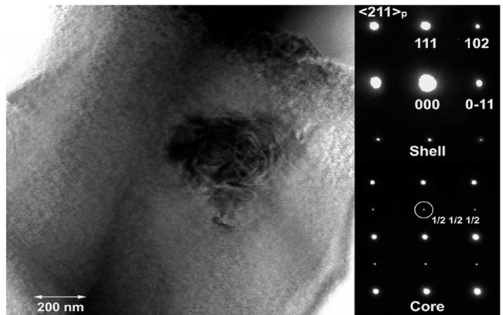
Figure 9. Bright field TEM image of 0.05\text{Bi}(\text{Zn}_{2/3}\text{Nb}_{1/3})\text{O}_3 -doped BF–BT, and diffraction pattern in core and shell regions. Reprinted with the permission of [78]. Copyright © 2018 American Chemical Society.
