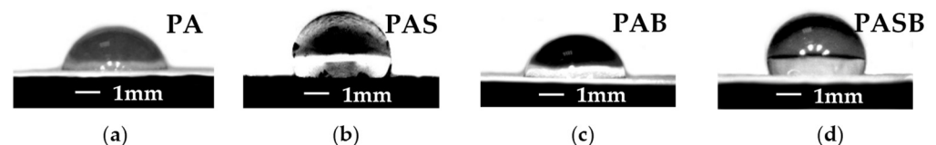
Figure 7. The surface contact angle measurements of samples (a) PA, (b) PAS, (c) PAB, and (d) PASB.
