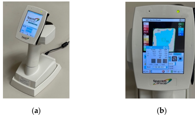
Figure 3. (a) Dental spectrophotometer and (b) its measurement screen.
