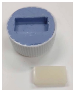
Figure 2. Silicone mold (20 mm (length) × 10 mm (width) × 4 mm (depth)) and resin block.
