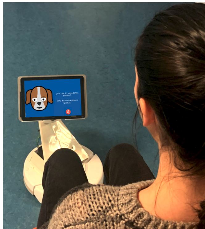
Figure 6. System appearance. The muted microphone under the text to the right of the avatar indicates the chatbot's turn to talk.
