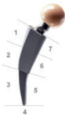
Figure 4. Metha Short Hip Stem prosthesis and definition of Gruen's periprosthetic zones.
