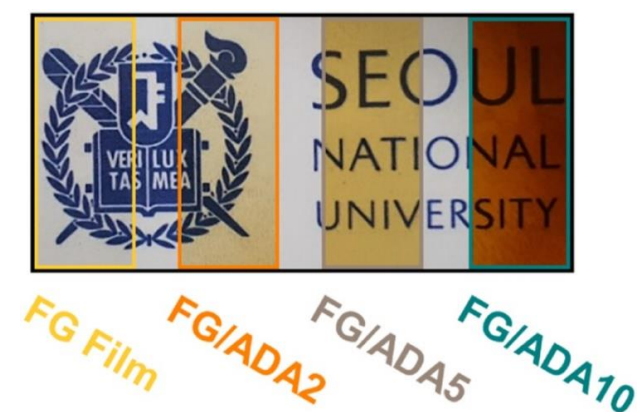
Figure 3. Optical properties of fish gelatin (FG)/alginate dialdehyde (ADA) composite films. Reproduced with permission from [13]. Copyright 2021 Elsevier.
